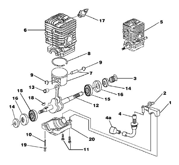
B2720 Chain Saw UT-10875 Engine Internal - Oil Pump Page 10 of 14
