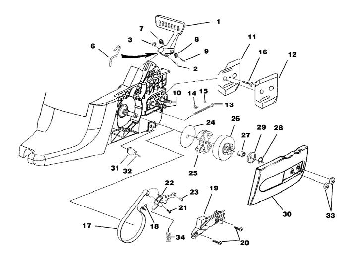
27av w/cc Chain Saw UT-10863 Clutch - Chain Brake - Drive Case Cover Page 6 of 14
