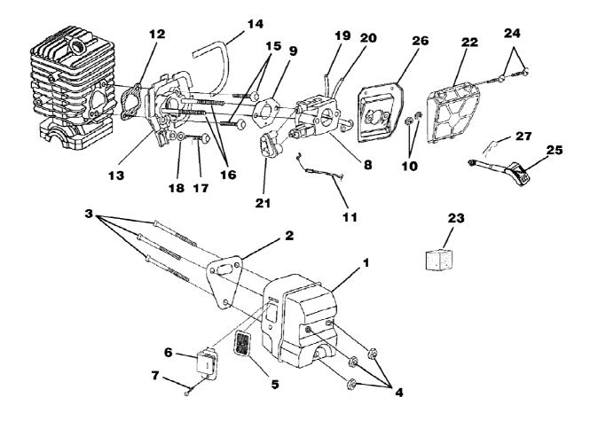
27av w/cc Chain Saw UT-10863 Carburetor - Muffler - Air Filter Page 4 of 14
