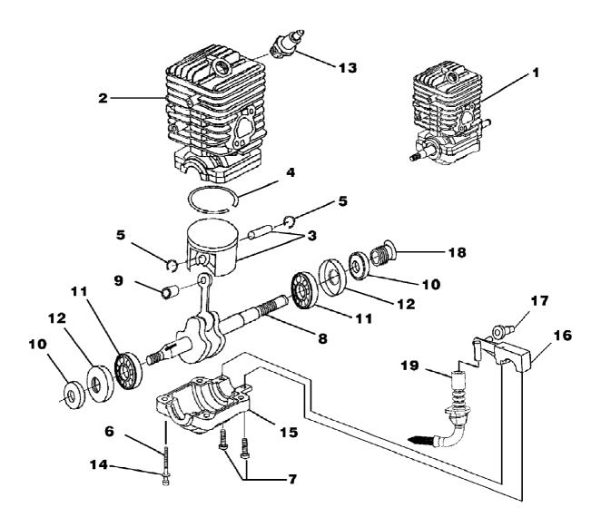
27av w/cc Chain Saw UT-10848 Engine Internal - Oil Pump Page 10 of 14
