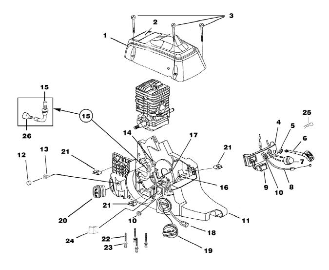
27av w/cc Chain Saw UT-10825 Engine Housing - Fuel Tank - Oil Tank Page 8 of 14
