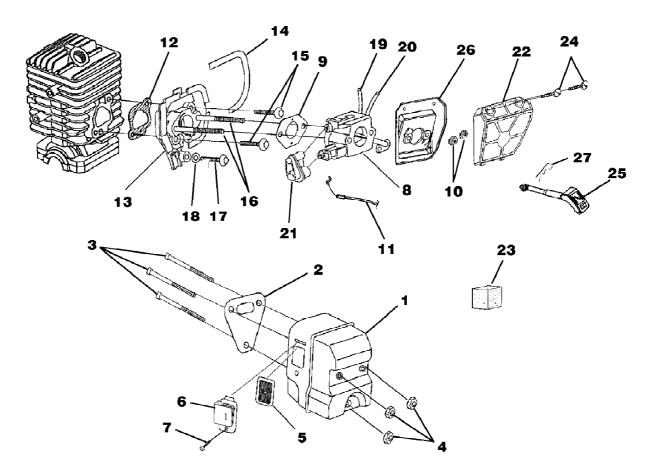
27av Chain Saw UT-10874 Carburetor - Muffler - Air Filter Page 4 of 14
