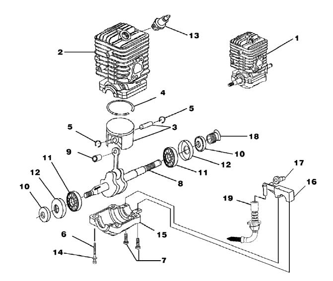
27av Chain Saw UT-10874 Engine Internal - Oil Pump Page 10 of 14
