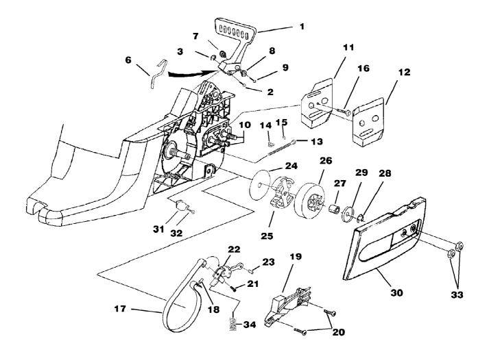
27av Chain Saw UT-10874 Clutch - Chain Brake - Drive Case Cover Page 6 of 14
