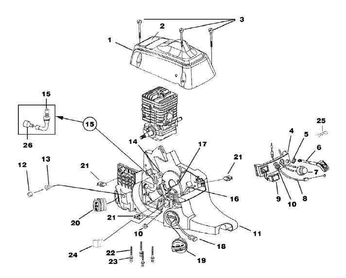
27av Chain Saw UT-10859 Engine Housing - Fuel Tank - Oil Tank Page 8 of 14
