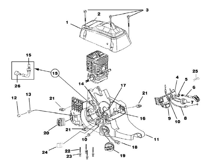
23av w/cc Chain Saw UT-10888 Engine Housing - Fuel Tank - Oil Tank Page 8 of 14
