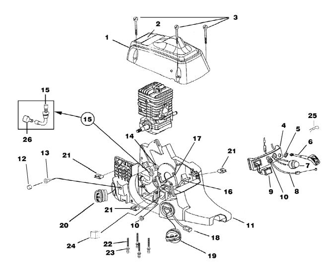
23av w/cc Chain Saw UT-10823 Engine Housing - Fuel Tank - Oil Tank Page 8 of 14
