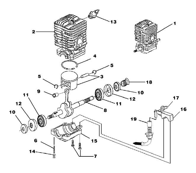
23av Chain Saw UT-10846 Engine Internal - Oil Pump Page 10 of 14
