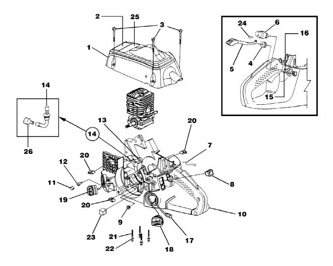
23 w/cc Chain Saw UT-10785-A Engine Housing - Fuel Tank - Oil Tank Page 8 of 14
