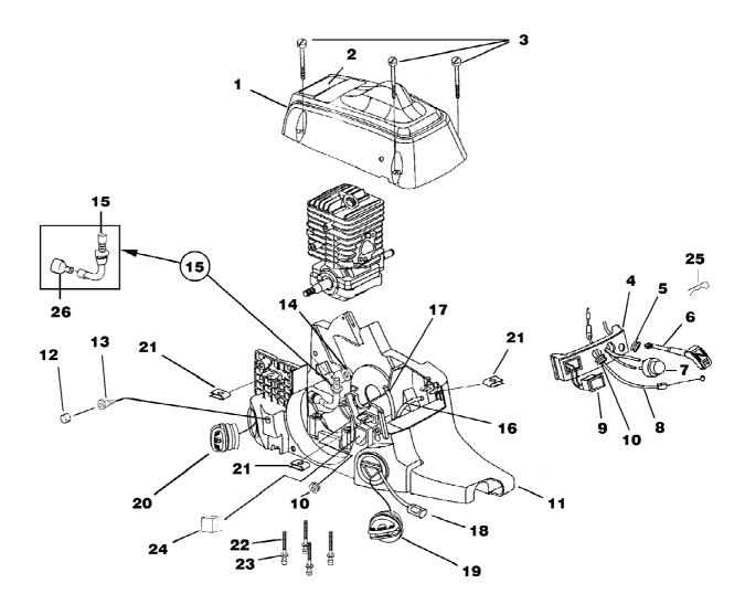
20av Chain Saw UT-10759-A Engine Housing - Fuel Tank - Oil Tank Page 8 of 14
