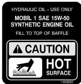
PART NO. 1-523552 LOCATION: Top Surface of Hydraulic Tank
