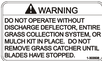
PART NO. 1-303508 LOCATION: On Top Rear Right Hand Surface of Mower Deck
