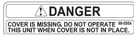
PART NO. 98-5954 LOCATION: - Under LH and RH Belt Shields - Radiator Fan Pump Idler Arm
