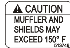
PART NO. 1-513746 LOCATION: On Engine Blower Housing next to Muffler & on Center Belt Cover
