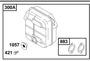
NOTE: This muffler is intended for replacement purposes only and is not to be used for retrofitting to engines with different exhaust systems.
