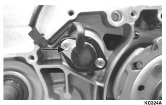
12. Remove the gear position switch. Account for a spacer.
