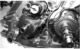
8. Align the shift forks to allow engagement with the shift cam; then engage the shift forks and slide the shift fork shaft into the locating boss in the crankcase.
