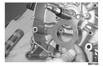
Installing Left-Side Components
