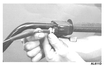
2. Turn the adjuster until the throttle cable has proper free-play of 3-6 mm (1/8-1/4 in.) at the lever.
