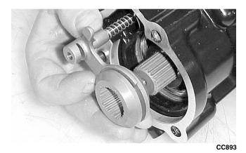
6. Place the input shaft assembly onto the gear case housing; then secure with the existing cap screws. Tighten to 18 ft-lb.
