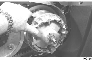
3. With two drops of red Loctite #271 on the threads and with the splines of the clutch shaft protruding through the movable drive face, install the nut and tighten to 147 ft-lb.
