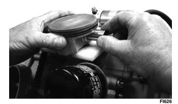
■NOTE: The piston should be installed so the IN points towards the intake side.
