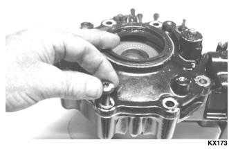
3. Using a plastic mallet, tap lightly to remove the differential cover. Account for an O-ring and a shim.
