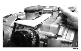
14. Using Piston Pin Puller, remove the piston pin. Account for the opposite-side circlip. Remove the piston.
