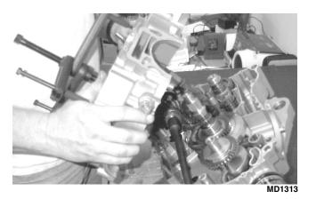
Disassembling Crankcase Half
