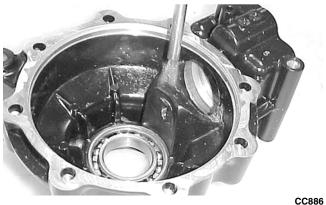
3. Using a flat-nosed punch, drive the bearing out of
