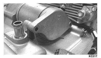
Remove starter motor by tapping lightly with a mallet.
