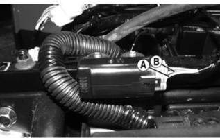
4. Tilt the sensor 60° or more to the left and right observing the meter. The meter should read 3.0-7.0 DC volts after approximately one second in the tilted position. If the meter readings are not as specified, the tilt sensor is defective.
