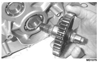
2. Install and tighten the output shaft flange nut to 59 ft-lb. Using a punch, peen the nut.
