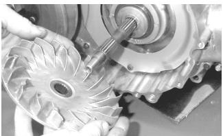
7. Remove the nut holding the driven pulley assembly; then remove the driven pulley assembly; mymowerparts.com
