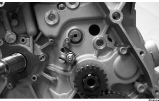
13. Remove the snap ring securing the output drive gear to the output shaft and remove the gear noting that the hub flange is directed toward the crank-
