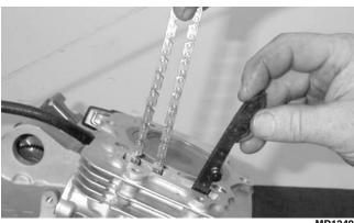
6. Place a new gasket into position on the cylinder. Place the alignment pins into position; then place the head assembly into position on the cylinder making sure the cam chain is routed through the chain cavity.
