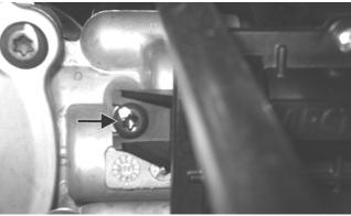
4. Loosen the front cap screw; then tighten the cap screw on the driveshaft side.
