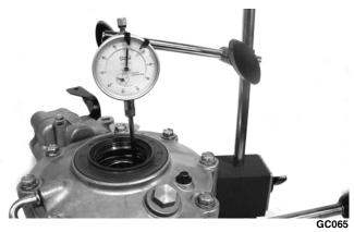
2. Zero the dial indicator; then push the ring gear toward the dial indicator and release. End-play should be 0.004-0.008 in.
