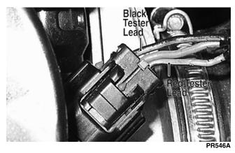
8. Select the DC Voltage position on the meter and turn the ignition switch to the ON position. The meter should read approximately 4.5 DC volt with the throttle closed and approximately 1.5 DC volts with the throttle in the full-open position.
