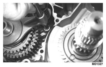
5. Remove snap ring and gear from the output side of the gear cluster. Remove the gear cluster and the inner shift fork together. Account for snap ring, gear, and washer.
