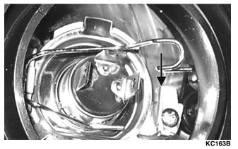
5. Connect the wiring harness connector to the bulb; then install the protective rubber boot making sure it seals completely on the headlight harness.
