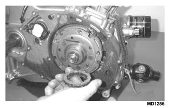
7. Install gear position switch spacer and switch making sure to align the drive pin with the slot in the shift shaft.
