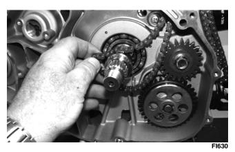
14. Remove the oil pump drive gear cap screw.
