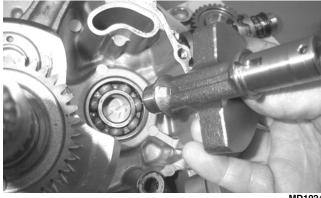
7. Using Crankcase Separator/Crankshaft Remover with the appropriate crankshaft protector, remove the crankshaft.
