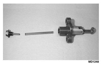
22. Depress the spring-loaded lock and push the plunger into the tensioner.
