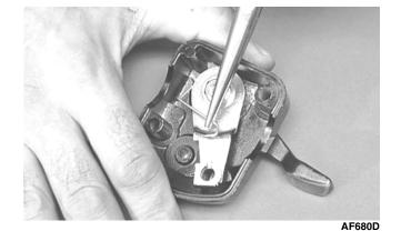
3. Place the two halves of the throttle control onto the handlebar and secure with the two machine screws.
