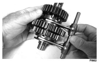
■NOTE: The countershaft assembly is now ready to be installed.
