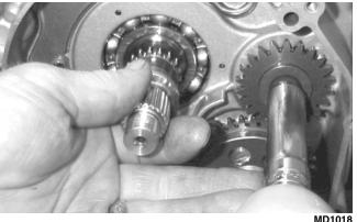
17. Remove oil pump drive gear. Account for the pin.
