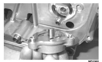
2. Place the thrust washer and drive pin into position on the oil pump shaft, install the oil pump driven gear making sure the recessed side of the gear is directed inward, and secure with a new snap ring.
