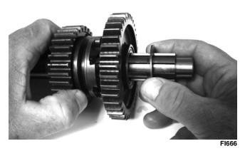
4. Place the reverse driven bushing (13) onto the shaft; then install the bearing (14), gear (15), and splined washer (16). Secure with a snap-ring.
