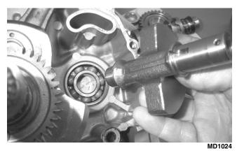
9. Using Crankcase Separator/Crankshaft Remover, remove the crankshaft.
