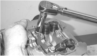
8. Install the two lower nuts securing the cylinder head to the cylinder, one in front and one in rear.
