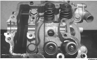
10. Remove the cylinder head from the cylinder, remove the gasket, and account for two alignment
