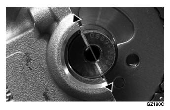
■NOTE: When the camshaft assembly is seated, make sure the alignment pin in the camshaft aligns with the smallest hole in the sprocket.
