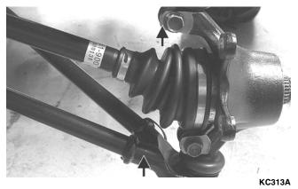
3. Install the tie rod end and secure with the nut. Tighten to 30 ft-lb; then install a new cotter pin and spread the pin.
