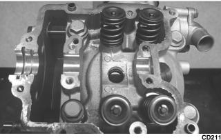
9. Remove the cylinder head from the cylinder, remove the gasket, and account for two alignment
