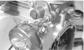
24. Install the cap screw and spring into the end of the cam chain tensioner. Tighten securely.
