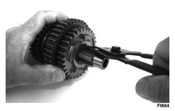
5. Install the reverse dog on the shaft; then place the shift forks and shift shaft into position.
