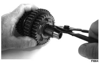
2. Remove the splined washer; then remove the reverse driven gear along with the bearing and bushing.
