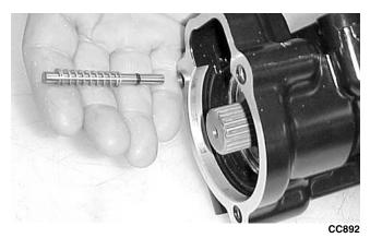
5. Install the shift fork assembly making sure the fork leg is facing upward. Apply a small amount of oil to the gasket; then install the gasket (425).
