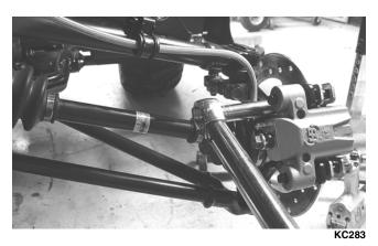
6. Tighten the hub nut (from step 4) to 200 ft-lb; then install and spread a new cotter pin making sure www.mymowerparashcoiden of the pin is flush to the hub nut.
