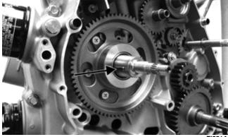
8. Install the rotor/flywheel and secure with the flange nut. Tighten to 107 ft-lb.
