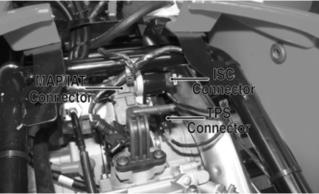
4. Remove the throttle arm cover and loosen the throttle cable jam nut; then disconnect the throttle cable and remove the throttle body.
