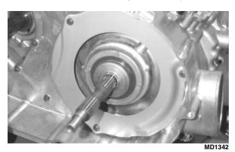
11. Place the driven pulley assembly into position and secure with the nut (threads coated with red Loctite #271). Tighten to 147 ft-lb.
