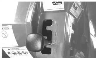
With the engine stopped and the brake lever lock engaged, turn the ignition switch to the ON position; then shift the transmission into each of the gear positions and note that the gear position indicated on the LCD corresponds to the gear position selected by the lever.
