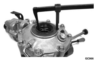
2. Using a press, remove the bearing.
