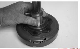
3. Check that the clutch shoe can only be rotated counterclockwise in respect to the clutch housing. If the clutch shoe locks up or turns in both directions, the one-way clutch must be replaced.
