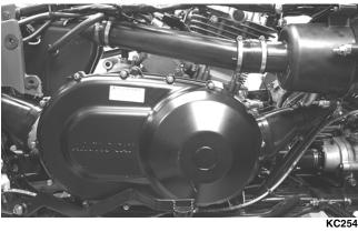
9. Install the shift rod onto the shift arm with bushing and flat washer and secure with an E-clip; then connect the speedometer sensor plug.
