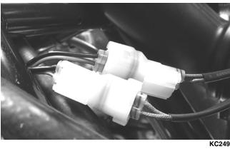
4. Disconnect the speedometer sensor; then remove the E-clip securing the shift rod to the shift arm and disconnect the shift rod. Account for a bushing and flat washer.
