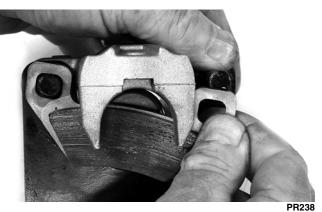
5. Remove the caliper holder from the caliper and discard the O-ring.
