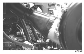
6. Remove the cap screws securing the exhaust pipe to the cylinder head; then disconnect the exhaust pipe to muffler springs and remove the exhaust pipe. Account for a grafoil seal and seal ring.
