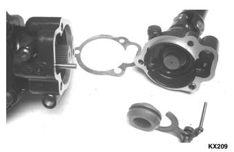
2. Remove the cap screws securing the gear case cover. Account for and make note of the ID tag location for assembling purposes.
