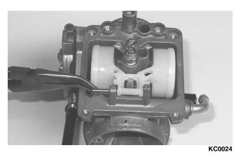
■NOTE: Check float height by placing the carburetor on its side w/float contacting the needle; then measure with a caliper the height when the float arm is in contact with the needle valve. Float arm height should be 17 mm.
