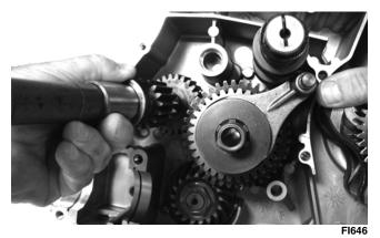
10. Install the spacer (1), shaft (2), reverse idler gear, and washer (3).
