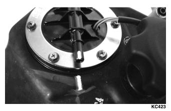
5. Disconnect the gas line connector from the fuel pump outlet.
