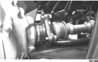
3. Remove the two cap screws and lock nuts securing the rear gear case to the frame; then remove the gear case through the left side.
