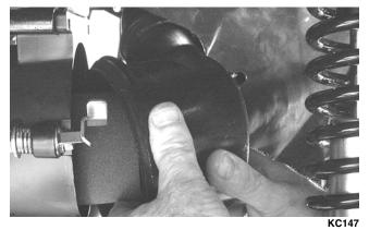
2. Remove the foam filter element from the air filter housing and separate the foam element from the spring.
