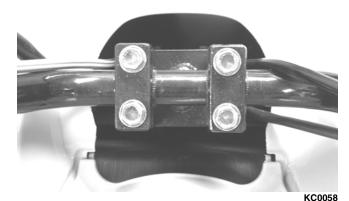
3. Remove the cap screws securing the upper steering post to the frame. Account for the housing cap, outer housing, and inner housing.
