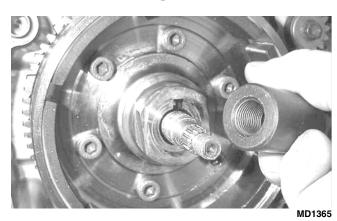
6. Using Magneto Rotor Remover, break the rotor/flywheel assembly loose from the crankshaft. Remove the remover, the crankshaft protector, the rotor/flywheel, and the starter clutch gear. Account for the key.
