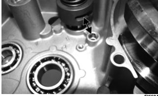
7. Place the shift forks into position on the assembled countershaft and install into the crankshaft as an assembly.
