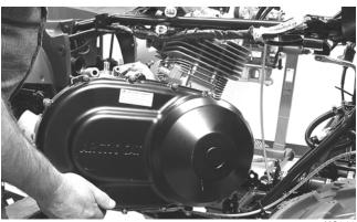
2. Install the front and rear engine mounting through-bolts and secure with the flange nuts. Tighten to 38 ft-lb.
