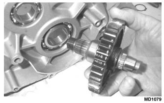
2. Apply red Loctite #271 to the threads of the output shaft. Install and tighten the nut 59 ft-lb. Using a punch, peen the nut.
