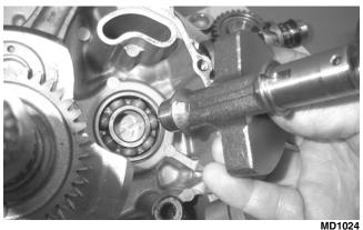
5. Install the key in the crank balancer shaft; then install the gear and aligning the timing marks, slide the gear into place.
