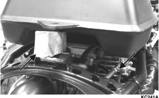
3. Remove all blocking and secure the gas tank with the cap screw. Tighten securely; then connect the gasline connector to the fuel pump outlet (425).
