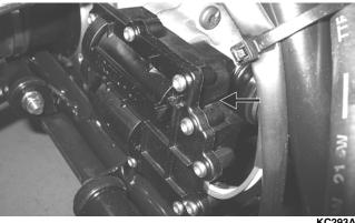
3. Remove the mounting cap screw from below the actuator on the suspension side.
