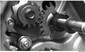
12. Remove the shift detent cam arm and spring.
