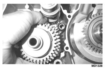
6. Noting the position of the slot on the end, remove the shift cam assembly. Account for inner and outer washers.
