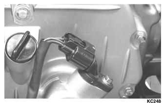
10. Connect the oil temperature connector and cooling fan connector; then using new O-rings, install the oil fittings onto the crankcase and secure with the cap screws. Tighten to 8 ft-lb.
