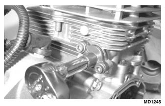
4. Remove the cam chain tensioner pivot cap screw and washer.
