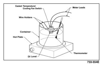
3. On the coolant temperature switch when the oil temperature reaches 112-118° C (234-244° F), the meter should show a closed circuit.
