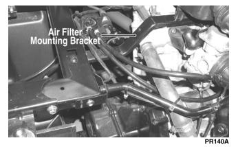
10. Remove the throttle arm cover from the carburetor/throttle body; then disconnect and remove the throttle cable and the carburetor/throttle body.
