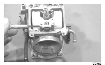
6. Lift the float assembly from the carburetor. Account for the float valve.
