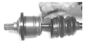
7. Slide the boot over the housing; then using the www.wpphelawppheressecure the boot with the clamp.
