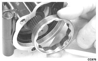
8. Using the Pinion Gear/Shaft Removal Tool and a hammer, remove the pinion gear from the gear case housing.
