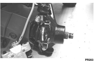
3. Install the tie rod end and secure with the nut (coated with red Loctite #271). Tighten to 30 ft-lb; then install a new cotter pin and spread the pin.
