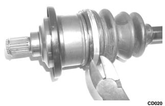
2. Wipe away excess grease to access the retaining ring. Using an awl or circlip pliers, remove the circlip.
