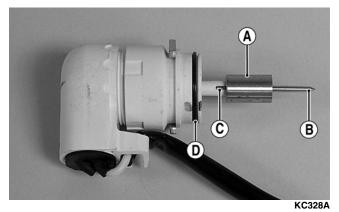
2. With the choke at room temperature (approximately 70° F), measure plunger extension. Measurement (A) should be 18.6-19.1 mm.
