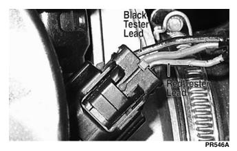
9. Select the DC Voltage position on the meter and turn the ignition switch to the ON position. The meter should read approximately 0.6 DC volts with the throttle closed and approximately 5.0 DC volts with the throttle in the full-open position.
