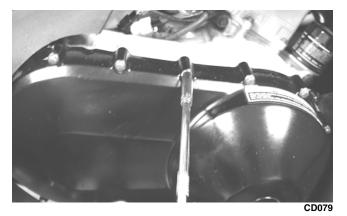
2. Remove the nut securing the movable drive face; then remove the face. Account for a flat washer and spacer.
