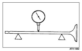
2. Maximum runout must not exceed specifications.
