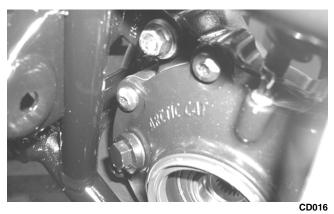
18. Free the differential assembly from the frame mountings; then lower the differential through the frame.
