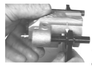
6. Plug the fluid port with a suitable plug to prevent contamination during cleaning.
