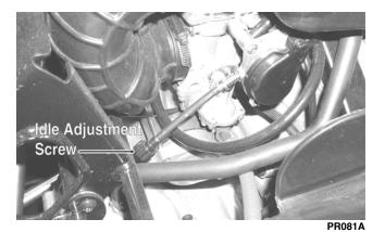
Adjust the idle to the correct RPM. Make sure the engine is at normal operating temperature before adjusting the idle RPM.
