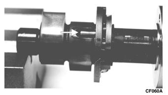
2. If damaged, the camshaft must be replaced.
