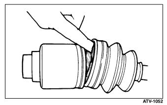
■NOTE: The grease pack contains 120 grams of grease. The inside joint (double-offset) requires
