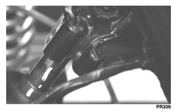
3. Apply green Loctite #270 to the cap screw; then secure the lower steering shaft joint to the pinion shaft making sure the shaft does not protrude into the joint beyond the clamping surface.
