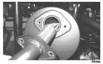
2. Using a suitable brush, clean the carbon deposits from the screen taking care not to damage the screen.
