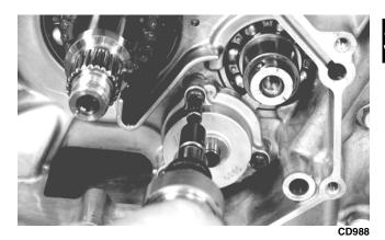
4. Install the oil pump drive gear spacer onto the crank balancer shaft. Grease the pin and insert it into the shaft; then install the drive gear making sure the raised side of the gear is facing toward the inside. Secure the gear with the cap screw (threads coated with red Loctite #271) and the washer. Tighten the cap screw to 62 ft-lb.
