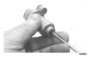
■NOTE: The adjuster shaft will be drawn into the tensioner as the adjuster screw is rotated clockwise. The adjuster shaft tension will be released in step 24.
