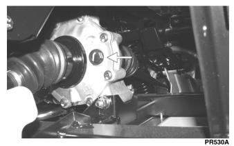
2. If low, add SAE approved 80W-90 hypoid gear lube as necessary.
