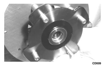
6. Secure the hub assembly with the nut. Tighten to 200 ft-lb.
