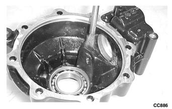
3. Using a flat-nosed punch, drive the bearing out of the housing.
