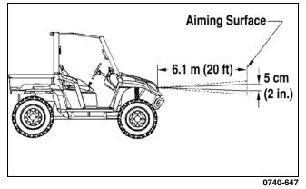
7. Using the adjuster knob, adjust each headlight until correct aim is obtained.
