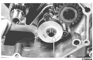
14. Remove the cap screws securing the oil pump; then remove the pump.
