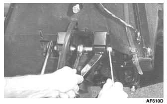
11. Remove the snap ring from the ball joint; then remove the ball joint from the A-arm.
