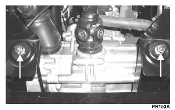
17. Remove two flange nuts securing the engine mounting bracket to the front engine mounts.
