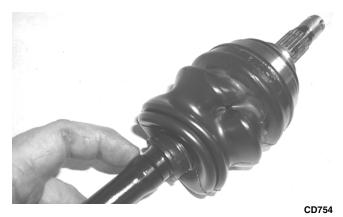
2. Using the boot clamp tool, secure the small clamp of the inner boot.
