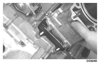
4. Loosely install the two nuts which secure the cylinder to the crankcase. ■NOTE: The two cylinder-to-crankcase nuts will be tightened in step 10.
