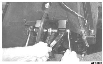
3. Route the brake hose through the upper A-arm shock absorber mount.
