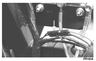
3. The meter must show less than 1 ohm.
