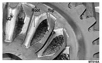
6. To adjust tooth contact, use the following chart to correctly shim the driven shaft.
