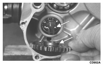
■NOTE: There is an oil passage beneath the driven gear/drive gear assembly. This passage should be plugged prior to removing the driven gear and
