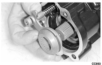
7. Place the input shaft assembly onto the housing; then secure with the existing cap screws. Tighten to 23 ft-lb.
