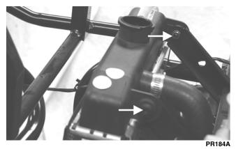
2. Connect the upper and lower coolant hoses to the radiator and secure with the appropriate hose clamps; then connect the cooling fan wire connector to the main harness.
