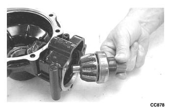
9. Secure the pinion gear in a bearing puller; then remove the pinion bearing using a press. Account for a collar and a bearing.
