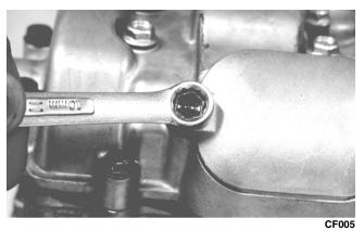
9. Install the spark plug; then install the timing inspection plug.
