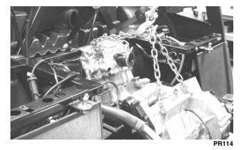
■NOTE: The front engine mounting bracket should slide free of the engine mounts first; then the rear engine mounting bracket and two rear engine mounts will lift free of the frame.
