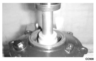
3. Using a press, install the new bearing into the housing.
