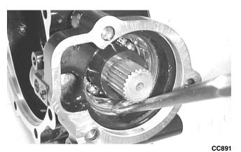
5. Install the pinion housing.
