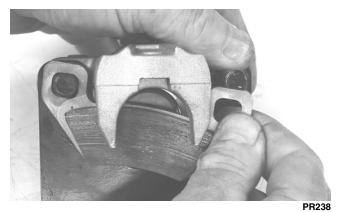
5. Remove the caliper holder from the caliper and account for the brake caliper O-ring. Do not remove the piston from the caliper.
