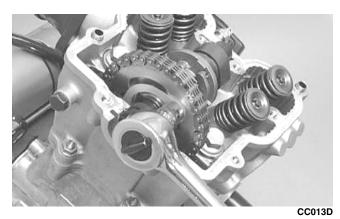
6. Remove the cap screw securing the chain tensioner (account for a washer); then remove the tensioner.
