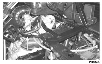
8. Loosen the clamp (A) securing the air intake boot to the carburetor/throttle body and the clamp (B) securing the air filter housing to the inlet housing boot; then remove the crankcase breather hose from the crankcase.
