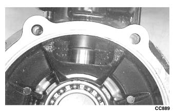
3. Install the pinion shaft and secure with the existing 48 mm lock collar. Tighten to 125 ft-lb.
