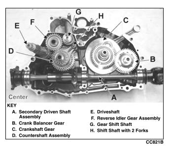
■NOTE: To aid in installing, it is recommended that the assemblies are kept together and IN ORDER.
