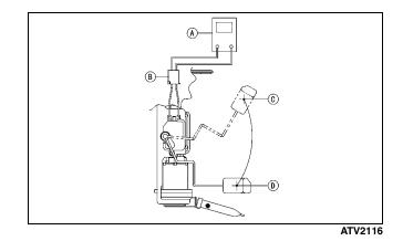
■NOTE: If readings are erratic, clean the resistor wiper and resistor with a clean cloth soaked with alcohol and retest. If the readings shown are not as specified, replace the fuel level sensor assembly.
