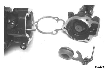
2. Using a T-40 torx wrench, remove the cap screws securing the differential cover. Account for and make note of the ID tag location for assembling purposes.
