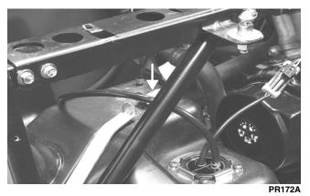
2. Swing the front hold-down to the right into position and install the cap screw and nut. Do not tighten at this time.
