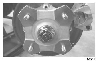
4. Slide the hub out of the knuckle and set aside.
