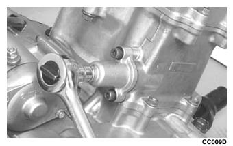
4. Using an awl, rotate the C-ring in its groove until it is out of the cylinder head; then remove the C-ring.
