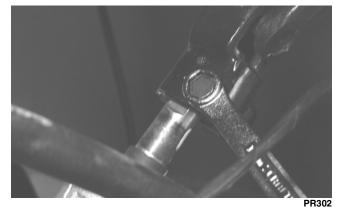
5. Remove two cap screws securing the rack and pinion assembly to the frame. Account for two nuts and two washers.
