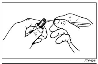
Before removing the spark plug, be sure to clean the area around the spark plug. Dirt could enter engine when removing or installing the spark plug.
