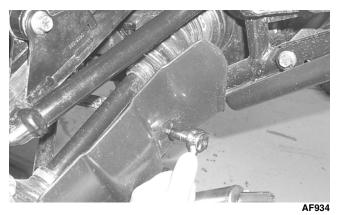
7. Slide the axle out of the knuckle and set aside.
