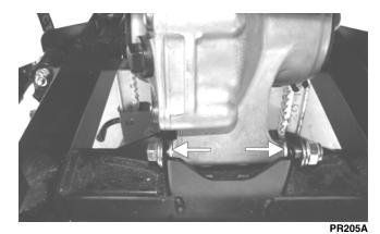
17. Remove the upper differential mounting cap screw. Account for a lock nut and two washers.
