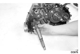
6. Place a washer on each end of the countershaft assembly; then install the assembly.
