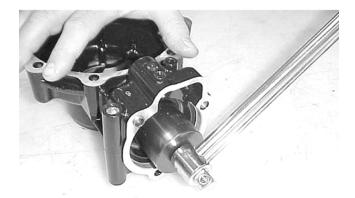
4. Place a punch on the edge of the lock collar in the oil gallery area; then using a hammer, stake the lock collar to ensure that the collar will remain securely tightened.
