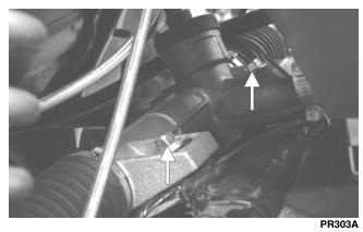
6. Remove the rack and pinion assembly from the right-side.
