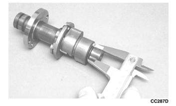
■NOTE: If the journals are worn, replace the camshaft; then measure the clearance again. If it is still out of tolerance, replace the cylinder head.
