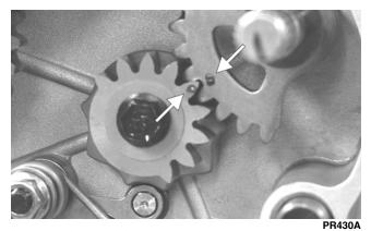
15. Remove the gear shift cam plate; then remove the shift cam stopper and cam stopper spring. Account for two washers.
