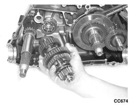
■NOTE: Do not disassemble the countershaft assembly unless necessary. If necessary, see Servicing Center Crankcase Components sub-section. 6. Using a rubber mallet, tap on the crankcase to remove the driveshaft (E).
