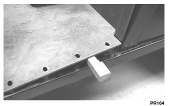
4. From the opposite side of the vehicle repeat step 3; then lift the rear of the floor up and lift the floor out of the vehicle.
