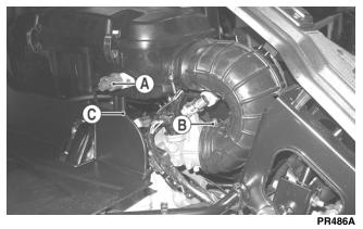
4. Disconnect the crankcase breather hose from the air filter housing; then remove the air filter assembly from the vehicle.
