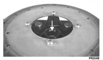
3. Install the hub assembly onto the axle; then set the parking brake.
