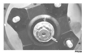
5. For front hubs, secure the brake calipers to the knuckle with two cap screws tightened to 20 ft-lb.
