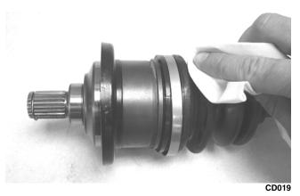
2. Inspect boots for any tears, cracks, or deterioration.
