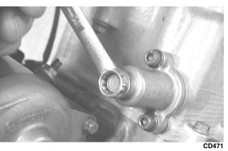
25. Loosen the four adjuster screw jam nuts; then loosen the four adjuster screws on the rocker arms in the valve cover.
