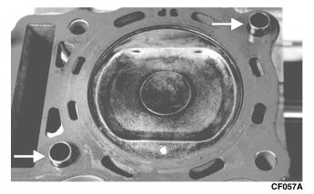
8. Install the four cylinder head cap screws. Tighten only until snug.
