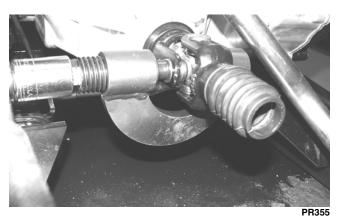
5. Check that the universal joint can be flexed freely without binding; then apply multi-purpose grease to the splines and install the propeller shaft noting the match marks made prior to removing.
