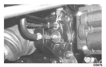
2. Turn the ignition switch to the ON position. The meter must show 12 DC volts.
