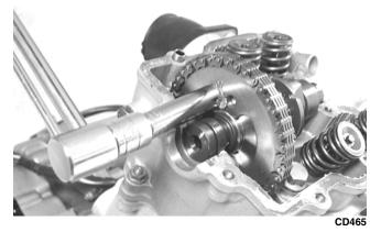
19. Rotate the crankshaft until the first cap screw (from step 17) can be addressed; then tighten to 11 ft-lb. Bend the tab to secure the cap screw.
