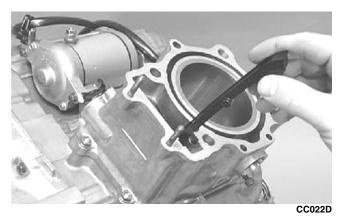
7. Place the head gasket into position on the cylinder. Place the alignment pins into position; then place the head assembly into position on the cylinder.
