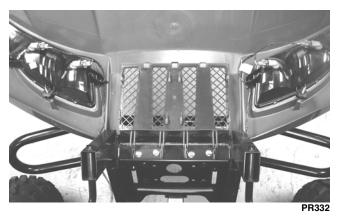
3. Connect the four headlight connectors; then secure the wires with two new nylon ties.
