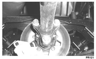
4. Install U-Joint Separator Tool on the universal joint fixed yoke; then remove the bearing cup retainers.
