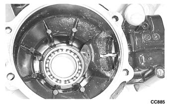
2. Using a propane torch, heat the area surrounding the needle bearing to soften the Loctite.
