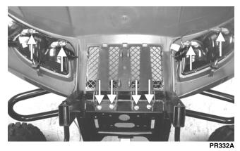
3. Finish removing the cap screws and flange nuts (from step 2); then remove the hood assembly.
