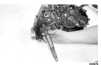
7. Note the timing marks on the crank balancer gear (B) and crankshaft gear (C) for assembling purposes; then slide the crank balancer gear off the crank balancer. Account for the key in the keyway.
