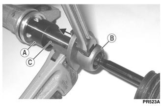
3. Clean all Loctite from the threads in the rack and if the tie rod is to be reused, clean the tie rod threads also.
