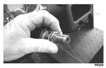
■NOTE: Some models have a castle nut/cotter pin and drilled steering shaft. Never reuse a cotter pin.
