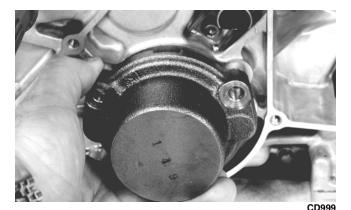
3. Install the oil pump onto the engine; then tighten the cap screws securely.
