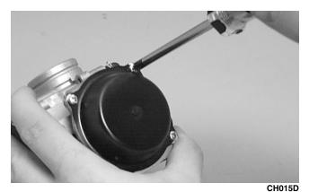
2. Remove the vacuum piston assembly from the carburetor body. Account for a spring, spring seat, and the jet needle.
