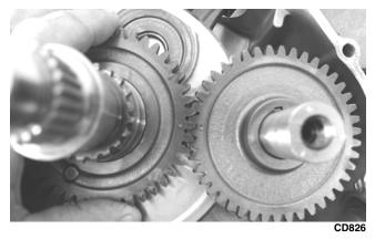
8. Remove the crank balancer.
