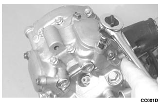
32. If removed, install the spark plug. Tighten securely.
