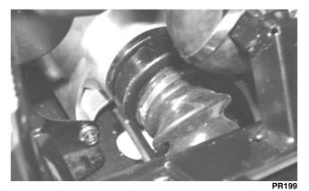
16. Remove the lower differential mounting cap screw. Account for a lock nut and four washers. Note the position of the washers for assembling.
