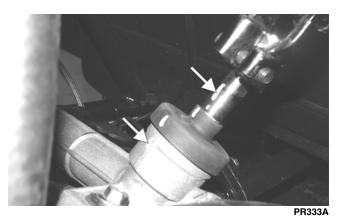
3. Apply green Loctite #270 to the cap screw; then secure the lower steering shaft joint to the pinion shaft making sure the pinion shaft does not pro-trude into the joint beyond the clamping surface. Tighten to 36 ft-lb.
