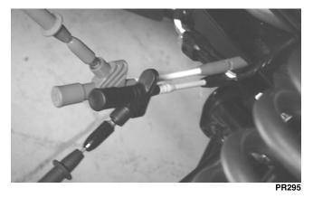
■NOTE: The black tester lead can remain connected to the black wire for the remaining tests.
