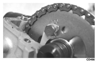
20. Place the C-ring into position in its groove in the cylinder head.
