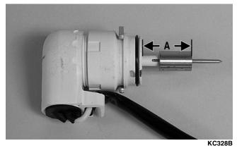
3. Connect Electric Choke Test Harness to the choke connector and a suitable 12 DC volt power supply for 2-3 minutes. Disconnect the power and measure plunger extension. Measurement (B) should be 22.1-23.4 mm.
