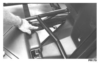
7. Remove four press-nuts securing the gas cap inset; then remove the gas cap and inset. Install the gas cap.
