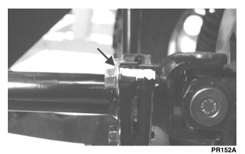
3. Remove the cap screws securing the propeller shaft flange to the yoke flange on the appropriate drive-line; then remove the propeller shaft.
