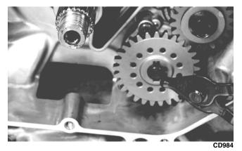
■NOTE: When installed correctly, the sides of the drive and driven gears will be flush with each other.
