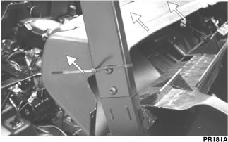
3. Remove the nuts securing the gauge assembly to the dash; then unplug the multi-pin connector and remove the gauge from the vehicle.
