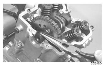
5. Bend the washer tabs down and remove the two cap screws securing the sprocket to the camshaft; then drop the sprocket off the camshaft.
