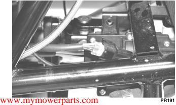
9. Remove two cap screws securing the differential lock cable support; then disconnect the differential lock cable at the differential.
