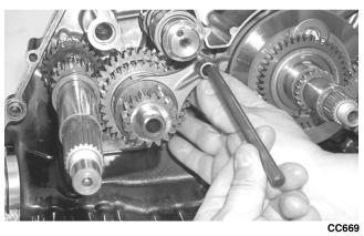
10. Install the reverse idler gear assembly noting the positioning of the two washers, gear, bushing, and shaft
