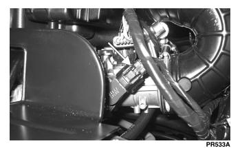
2. Remove the screw securing the TPS to the throttle body and remove the TPS.
