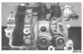
3. Loosen the cap screw on the end of the tensioner; then remove the two cap screws securing the tensioner adjuster assembly and remove the assembly. Account for a gasket.
