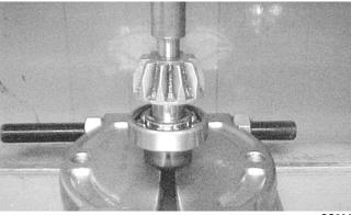
3. Install the pinion gear assembly into the housing. Using the 48 mm Internal Hex Socket, secure the pinion gear assembly with the existing lock collar. Tighten to 125 ft-lb.
