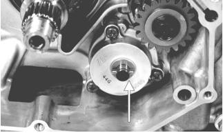
14. Remove the cap screws securing the oil pump; then remove the pump.
