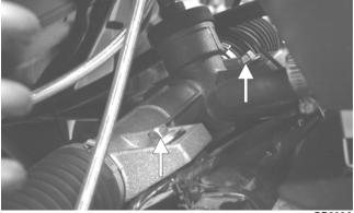
6. Remove the rack and pinion assembly from the right-side.
