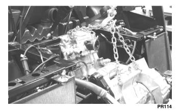
■NOTE: The rear engine mounting bracket and rear engine mounts should be attached to the engine. The front engine mounting bracket should be attached to the engine, and the front engine mounts should be in the frame.
