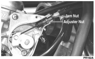
6. Disconnect the electric choke connector; then remove the carburetor from the engine.
