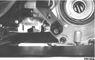
10. Remove the lower and upper ball joint cap screws taking care not to strip the threads on the ball joint shaft; then using a rubber mallet, tap the end of the axle and free it from the knuckle assembly.
