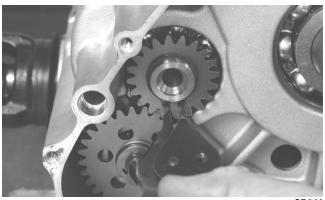
13. Remove the snap ring securing the water pump driven gear; then remove the gear noting the direction of the sides of the gear for installing purposes. Account for the driven gear alignment pin.
