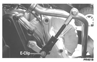
7. Remove four machine screws securing the shifter mount to the frame; then remove the shifter assembly.
