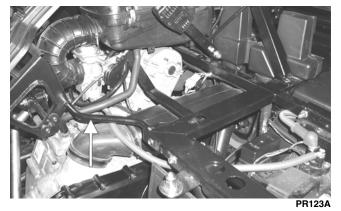
8. Loosen the clamp securing the air intake boot to the carburetor/throttle body and the clamp securing the air filter housing to the inlet housing boot; then remove the crankcase breather hose from the crankcase.
