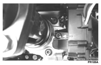
3. Remove the mounting cap screw from above the actuator on the suspension side.
