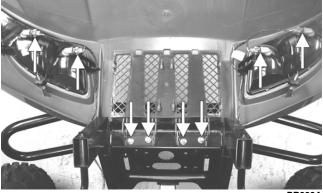
3. Finish removing the cap screws and flange nuts (from step 2); then remove the hood assembly.
