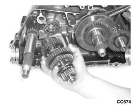
8. Place a washer on each end of the gear shift shaft; then install the shaft assembly making sure the two holes on the end of the shaft are positioned vertically.
