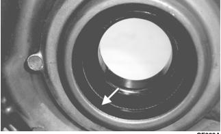
9. Remove the two Allen-head screws securing the gear shift position switch; then remove the sensor. Account for two neutral contact pins and two springs.
