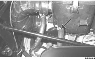
5. Slowly disconnect the gasline hose connector from the fuel rail.
