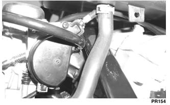
12. Place the air filter assembly into position and secure with the self-tapping screws; then connect the intake boot to the carburetor/throttle body and the inlet housing boot to the air filter housing. Tighten the clamps securely.
