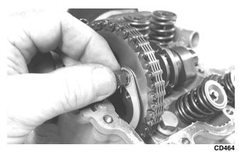
18. Rotate the crankshaft until the second cap screw securing the sprocket to the camshaft can be installed; then install the cap screw (threads coated with red Loctite #271) and tighten to 11 ft-lb. Bend the tab to secure the cap screw.
