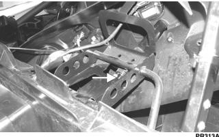
5. Apply green Loctite #270 to the cap screw; then install the cap screw in the upper steering shaft joint and finger-tighten.
