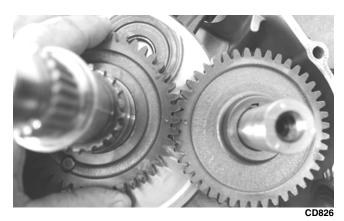
8. Remove the crank balancer.
