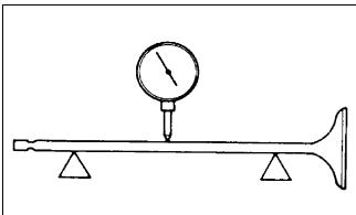
2. Maximum runout must not exceed specifications.
