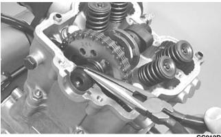
5. Bend the washer tabs down and remove the two cap screws securing the sprocket to the camshaft; then drop the sprocket off the camshaft.
