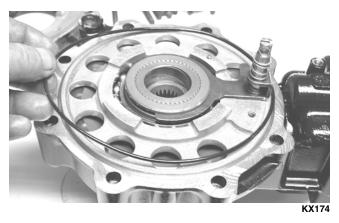
■NOTE: If the cover is difficult to remove, pry on the cover in more than one recessed location.
