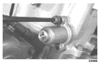
24. Using a flat-blade screwdriver, rotate the adjuster screw inside the tensioner counterclockwise until all tension is released; then install the cap screw into the end of the chain tensioner.
