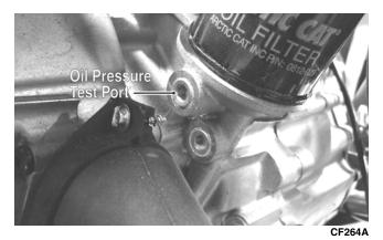
■NOTE: Some oil seepage may occur when installing the oil pressure gauge. Wipe up oil residue with a cloth.
