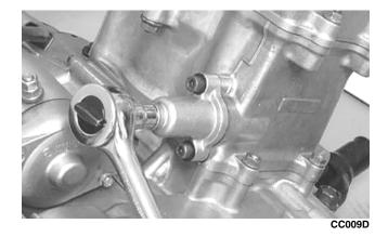
4. Using an awl, rotate the C-ring in its groove until it is out of the cylinder head; then remove the C-ring.
