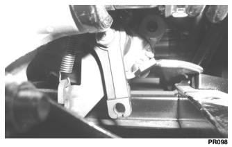
2. Rotate the actuator clockwise (hand tight) until it contacts the back of the piston; then rotate counterclockwise approximately one spline.
