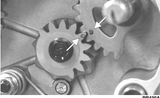
15. Remove the gear shift cam plate; then remove the cam stopper and cam stopper spring. Account for two washers.
