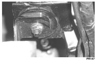
4. Apply multi-purpose grease to the driveshaft splines; then align the flange marks and slide the splines into the slip-joints.
