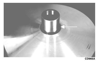
3. Remove the nut securing the fixed driven assembly; then remove the assembly.
