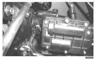
4. Loosen the front cap screw; then tighten the cap screw on the driveshaft side.
