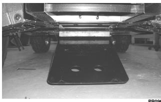
1. Remove the parking brake cable from the actuator lever; then remove the actuator nut and actuator lever. Note the position of the lever before removing.
