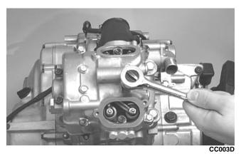
29. In a crisscross pattern starting from the center and working outward, tighten the cap screws securely.
