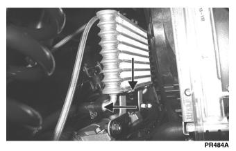
2. Remove the flange nuts and cap screws from the oil cooler mountings and remove the oil cooler.
