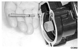
6. Install the shift fork assembly making sure the fork leg is facing upward. Apply a small amount of oil to the gasket; then install the gasket.
