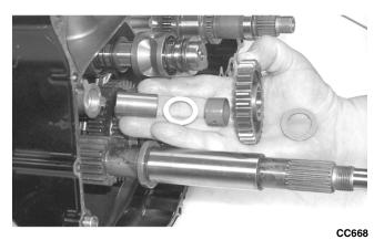
11. Install the front and rear secondary driven shaft assemblies into the left side of the crankcase making sure the bearing locating pins are facing upward and the bearing C-ring is fully seated in the crankcase.
