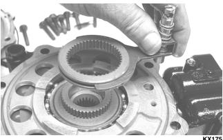
5. Remove the left gear case bearing flange assembly and account for a shim. Mark the shim as left-side.
