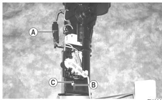
B. Engage the tabs (C) of the fuel level sensor into the mounting slot (B) and press toward the bottom of the fuel pump to latch in place; then connect the two-wire connector (A).
