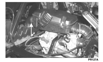
9. Remove four self-tapping screws securing the air filter mounting bracket to the frame; then remove the air filter and mounting bracket as an assembly.
