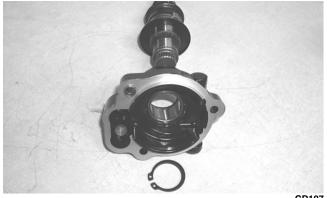
4. Using a seal removal tool, remove the input shaft seal. Account for a spacer.
