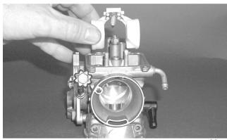
■NOTE: Check float arm height by placing the carburetor on its side w/float contacting the needle; then measure with a caliper the height when the float arm is in contact with the needle valve. Float arm height should be 17 mm (0.7 in.).
