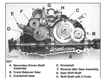
■NOTE: To aid in installing, it is recommended that the assemblies are kept together and IN ORDER.
