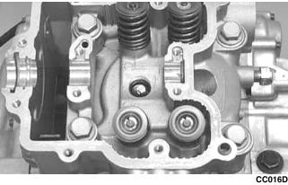
9. Remove the cylinder head from the cylinder, remove the gasket, and account for two alignment pins; then remove the cam chain guide.
