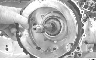
6. Remove the cap screws securing the clutch cover. Note the location of the different-lengthed cap screws for installing purposes. Using a rubber mallet, carefully remove the cover. Account for two alignment pins.
