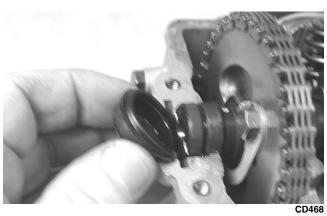
22. Remove the cap screw from the end of the chain tensioner; then using a flat-blade screwdriver, rotate the adjuster screw inside the tensioner clockwise until the screw bottoms.
