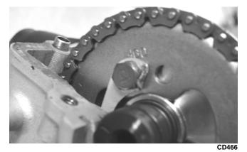
20. Place the C-ring into position in its groove in the cylinder head.
