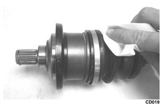
2. Inspect boots for any tears, cracks, or deterioration.
