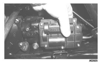
3. While holding the actuator firmly forward, tighten the front cap screw to hold the actuator in place; then install but do not tighten the two remaining cap screws.
