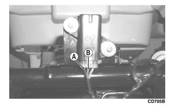
4. Tilt the sensor 60° or more to the left and right observing the meter. The meter should read 4.0-8.0 DC volts after approximately one second in the tilted position. If the meter readings are not as specified, the tilt sensor is defective.
