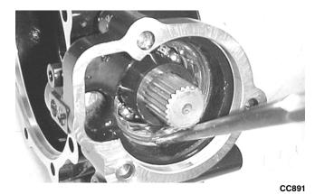
5. Install the pinion housing.
