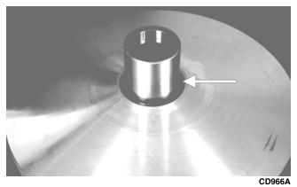
4. Install one of the V-belt cover cap screws into the driven pulley fixed face; then turn the cap screw clockwise to spread the pulley faces. Remove the V-belt.
