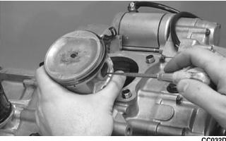
2. Place the two alignment pins into position. Place the cylinder gasket into position; then place a piston holder (or suitable substitute) beneath the piston skirt and square the piston in respect to the crankcase.
