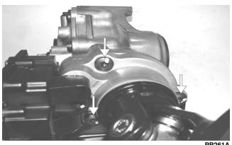
2. Using a rubber mallet, remove the housing. Account for a gasket. Remove the fork, collar, and spring. Note the location of all the components for assembling purposes.
