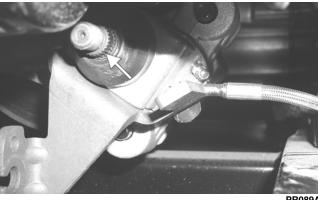
3. Install the actuator lever in the position noted in step 1; then install the actuator nut and tighten to 35 ft-lb.
