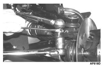
8. Apply grease to the hub and drive axle splines; then install the hub assembly onto the drive axle.
