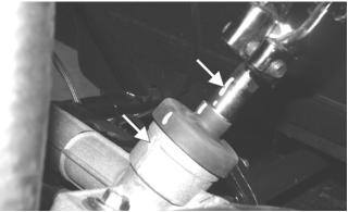
■NOTE: Any time steering components are disassembled, all connecting components should be marked for proper alignment during assembling.
