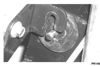
3. Install the flange nuts on the rear engine mount studs; then secure the front engine mounting bracket to the front engine mount studs with two flange nuts. Tighten the four flange nuts to 25 ft-lb.
