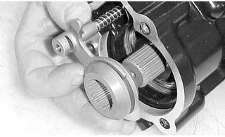
7. Place the input shaft assembly onto the gear housing; then secure with the existing cap screws. Tighten to 23 ft-lb.
