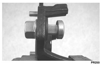
3. Using a socket and ratchet handle, tighten the nut until the stud is fully drawn into the hub.
