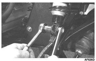
10. Remove the cap screws securing the A-arms to the
