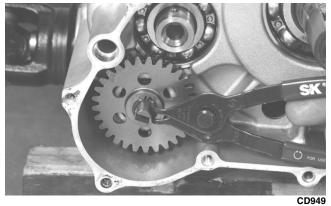
■NOTE: The sharp side of the snap ring should be facing outward.
