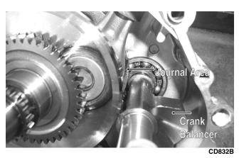
■NOTE: It will be necessary to rotate the crank balancer until the counterweight is facing away from the crankshaft; then rotate the crankshaft clockwise into the journal area to allow the crank balancer to be fully seated.
