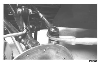
3. Make matching alignment marks on the pinion shaft and lower steering shaft joint.
