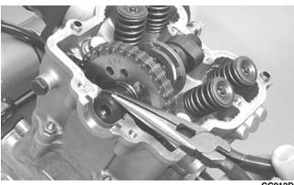
21. Install the cylinder head plug in the cylinder head with the open end facing downward and toward the inside.
