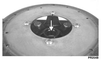
3. Install the hub assembly onto the axle; then set the parking brake.
