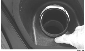
5. Secure the filler panel with four press-nuts; then tighten the hardware securing the hold-down straps (from steps 2-3) securely.
