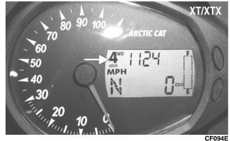
4. If the differential lock engages (front wheels locked) and the voltage does not drop to 0, the switch is faulty and must be cleaned or replaced.
