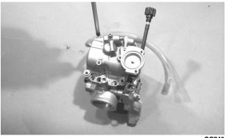
7. Place the U-ring into the pump housing. Position the spring and diaphragm assembly (lip toward the carburetor) onto the carburetor; then secure the assembly with the pump housing and three screws. Tighten securely.
