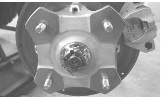
4. Slide the hub out of the knuckle and set aside.
