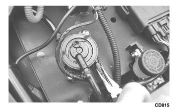
2. Start the engine. Fuel pump pressure should show 0.036-0.084 kg/cm<sup>2</sup> (0.5-1.2 psi).
