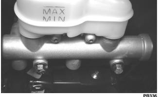
3. Remove the oil bolt securing the banjo-fittings to the master cylinder; then remove the master cylinder. Discard the three crush washers.
