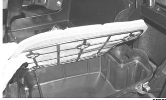
9. Install the air filter housing cover and secure with the retaining clips; then install the center console and seats making sure the seats lock securely.
