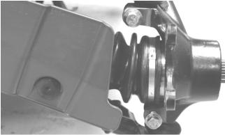
11. Pull the steering knuckle away from the axle taking care not to damage the seals with the axle end.
