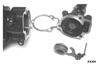
2. Using a T-40 torx wrench, remove the cap screws securing the gear case cover. Account for and make note of the ID tag location for assembling purposes.
