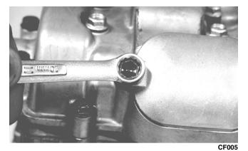
9. Install the spark plug; then install the timing inspection plug.
