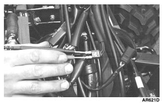
3. When the lever is depressed, the meter must show less than 1 ohm.
