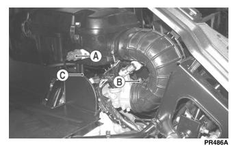
4. Disconnect the crankcase breather hose from the air filter housing; then remove the air filter assembly from the vehicle.
