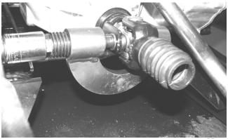
5. Check that the universal joint can be flexed freely without binding; then apply multi-purpose grease to the splines and install the propeller shaft noting the match marks made prior to removing.
