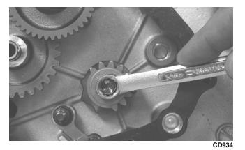
6. Install the shift cam stopper, spring, and two washers; then coat the threads on the mounting stud with red Loctite #271 and install the nut. Tighten securely.
