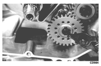
■NOTE: When installed correctly, the sides of the drive and driven gears will be flush with each other.
