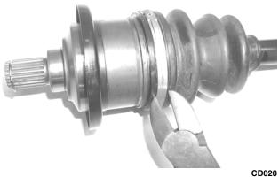
2. Wipe away excess grease to access the retaining ring. Using an awl or circlip pliers, remove the cir-
