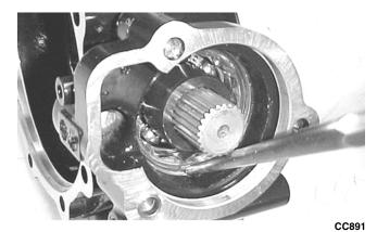
3. Note the following shim selections (shims are nominally 1.5 mm/0.060 in. thick):
