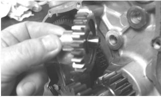
12. Remove the snap ring securing the water pump drive gear; then remove the gear noting the direction of the sides of the gear for installing purposes. Account for the drive gear alignment pin.
