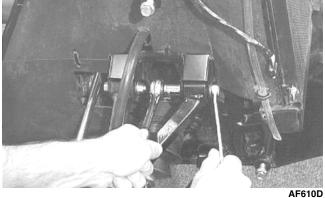
3. Route the brake hose through the upper A-arm shock absorber mount.
