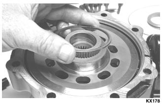
6. Place the differential with the open side down; then lift the housing off the spider assembly. Account for shim(s) and mark as right-side.
