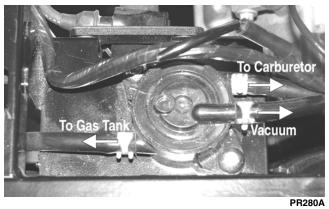
2. Remove the two machine screws and flange nuts securing the fuel pump to the electrical tray; then remove the pump.
