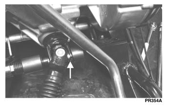
5. Using a suitable socket and ratchet handle, rotate the jackscrew to push the bearing cup out of the yoke; then remove the tool and the bearing cup.
