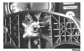
2. Remove the nut securing the steering wheel and remove the steering wheel. Account for the flat thrust-washer and two wave washers.
