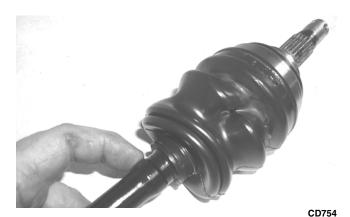
10. Using CV Boot Clamp Tool, secure both outside boot clamps.
