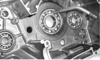
■NOTE: If heating the bearing is not possible, the crankshaft can be installed using a crankshaft installing tool.
