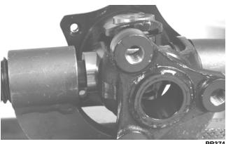
3. Install the retainer in the bearing cup; then remove the yoke from the separator tool.
