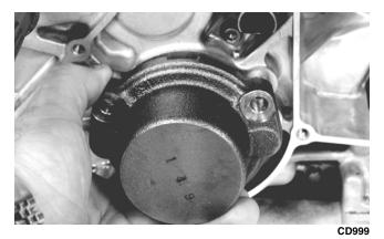
3. Install the oil pump onto the engine; then tighten the cap screws securely.
