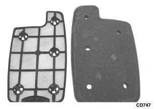
4. Fill a wash pan larger than the filter with a non-flammable cleaning solvent; then dip the filter in the solvent and wash it.
