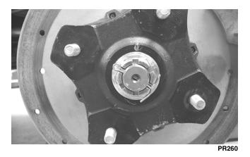
■NOTE: If the hole in the axle shaft does not align with the slots in the castle nut, tighten the nut until the hole and slots align.
