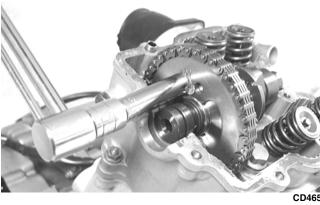
19. Rotate the crankshaft until the first cap screw (from step 17) can be addressed; then tighten to 11 ft-lb. Bend the tab to secure the cap screw.
