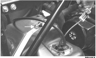
4. Place the gas cap filler panel into position; then if necessary, position the gas tank so the filler panel and filler neck are not binding or rubbing.
