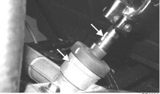
3. Apply green Loctite #270 to the cap screw; then secure the lower steering shaft joint to the pinion shaft making sure the pinion shaft does not protrude into the joint beyond the clamping surface. Tighten to 25 ft-lb.
