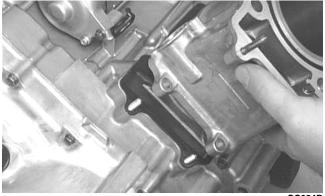
4. Loosely install the two nuts which secure the cylinder to the crankcase.
