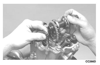
■NOTE: Loop the chain over the cylinder and secure it to keep it from falling into the crankcase.
