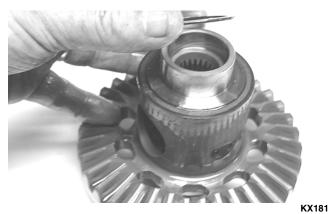
7. Using the 48 mm Internal Hex Socket, remove the lock collar securing the pinion gear assembly.
