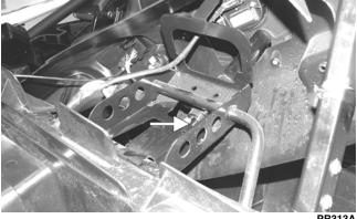
5. Remove the cap screw securing the lower steering shaft joint to the pinion shaft; then slide the steering shaft assembly free and remove through the opening in the splash panel.
