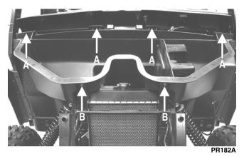
3. While lifting up on the front of the storage box, pry the rear center clear of the center dash mount and remove the storage box.
