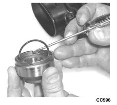
■NOTE: Account for and inspect the clutch housing seal.
