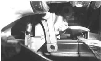
4. Install the parking brake cable and adjust nuts so the parking brake holds the vehicle when set and fully releases it when released.
