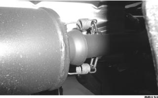
2. Slide the muffler assembly clear of the holder pins.
