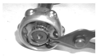
4. Note the difference inside each bearing ring end for assembling purposes; then remove the bearing ring.
