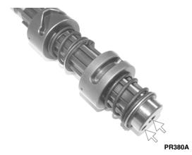
5. Remove the countershaft assembly (D). Account for a washer on each end of the countershaft.
