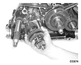
■NOTE: Do not disassemble the countershaft assembly unless necessary. If necessary, see Servicing Center Crankcase Components sub-section.
