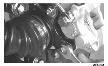
8. Disconnect the front drive actuator power connector from the main harness; then disconnect the differential lock indicator connector from the differential lock switch located on the right-side of the differential.
