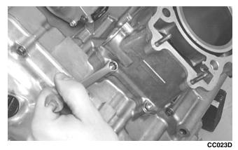
12. Lift the cylinder off the crankcase taking care not to allow the piston to drop against the crankcase. Account for the gasket and two alignment pins.
