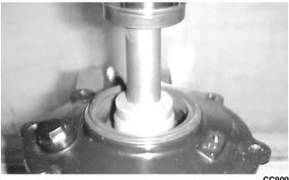
3. Using a press, install the new bearing into the housing.
