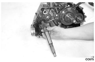
7. Place a washer on each end of the countershaft assembly; then install the assembly.
