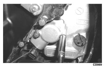
13. Place the water pump into position and secure with
