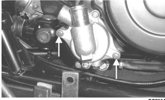
2. Connect the two coolant hoses to the water pump and secure with the clamps; then install the water pump coolant drain plug.
