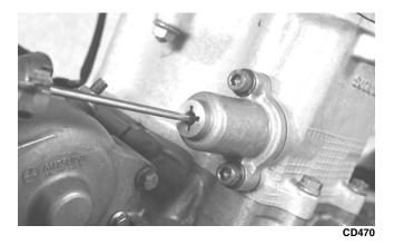
25. Loosen the four adjuster screw jam nuts; then loosen the four adjuster screws on the rocker arms in the valve cover.
