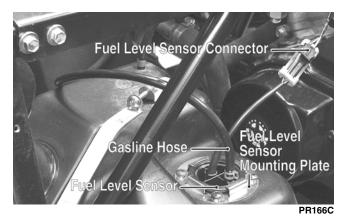
3. Remove the fuel level sensor from the gas tank. Account for a seal.
