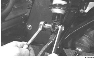
4. Using a suitable spring compression stand, compress the shock absorber spring, remove the retainer, and remove the spring.
