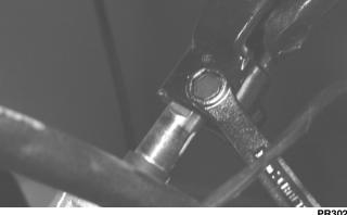
5. Remove two cap screws securing the rack and pinion assembly to the frame. Account for two nuts and two washers.
