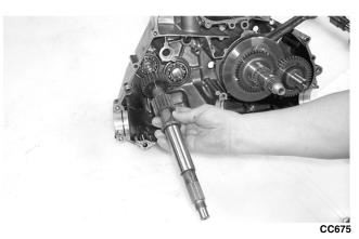
7. Note the timing marks on the crank balancer gear (B) and crankshaft gear (C) for assembling purposes; then slide the crank balancer gear off the crank balancer. Account for the key in the keyway.
