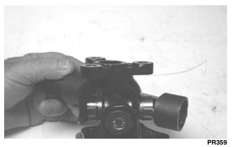
6. Install the separator tool on the opposite side of the yoke to push the second bearing cup from the yoke; then remove the tool and separate the universal joint.
