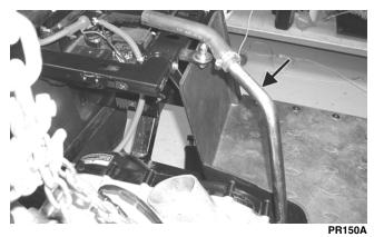
12. Remove the exhaust duct from the V-belt housing; then remove the inlet boot connecting the inlet duct to the V-belt housing.
