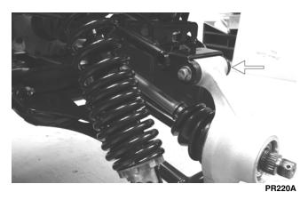
■NOTE: Never reuse a lock nut. Once a lock nut has been removed, it must be replaced with a new lock nut.
