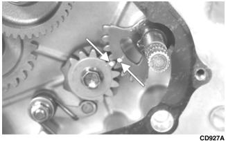
8. Lubricate the magneto cover gasket with fresh engine oil; then place it into position on the two alignment pins. Make sure the outer shift shaft washer is in place.
