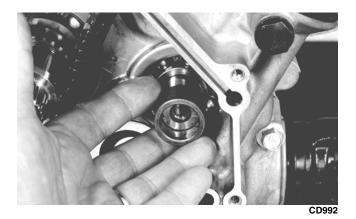
5. Grease the driven gear pin and insert it into the oil pump shaft; then install the driven gear (noting the direction of the sides of the gear from removing). Secure with a snap ring.
