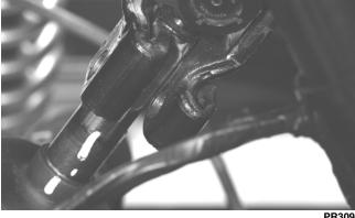
3. Apply green Loctite #270 to the cap screw; then secure the lower steering shaft joint to the pinion shaft making sure the shaft does not protrude into the joint beyond the clamping surface.
