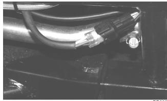
2. Connect the black lead to the black wire using a MaxiClip; then select 2WD on the 2WD/4WD selector switch.
