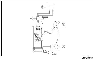
■NOTE: If readings are erratic, clean the resistor wiper and resistor with clean alcohol and retest. If still not correct, replace the fuel level sensor.
