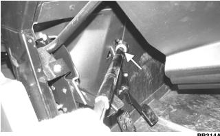
2. Align the match marks on the pinion shaft and the lower steering shaft joint; then slide the steering shaft joint onto the pinion shaft.
