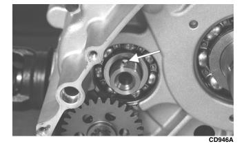
■NOTE: The sharp side of the snap ring should be facing outward.
