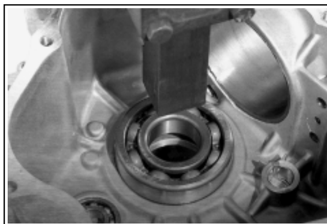
Figure 11-1. Installing Bearings Using a Press.
