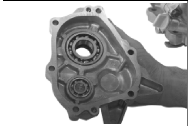
Figure 11-25. CS8.5-12. Installing Bearing.
