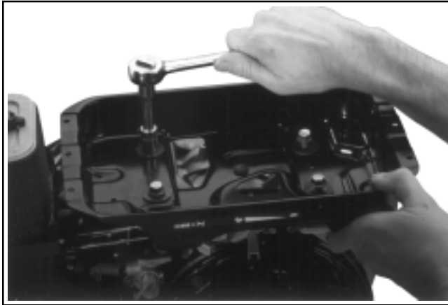
Figure 11-112. CS8.5 (spec. 95xxxx) Installing Fuel Tank Support.
