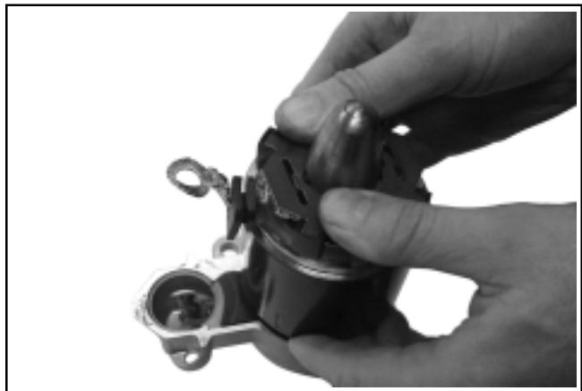
Figure 8-56. Installing Frame with Brush Plate Assembly.
