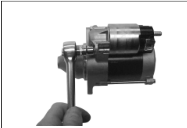
Figure 8-58. Installing Thru Bolts.
