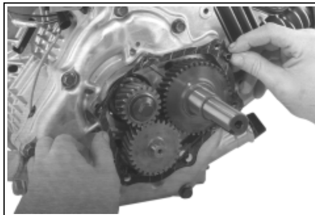
Figure 11-35. CS8.5-12. Installing Dowel Pins and Gasket.
