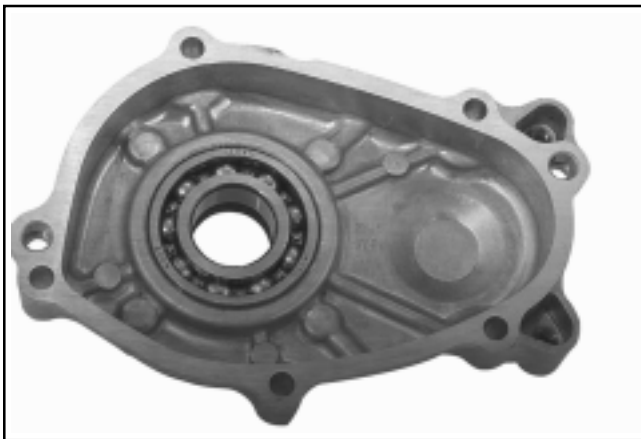
Figure 11-24. CS4, CS6. Installing Bearing.
