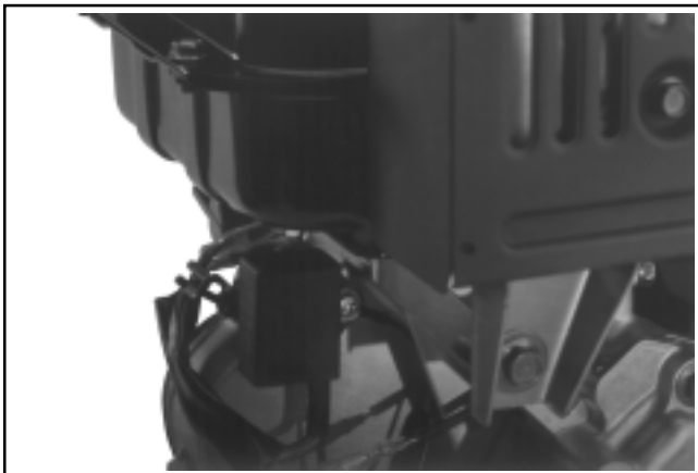
Figure 9-25. CS8.5 (spec. 95xxxx) Ground Lead Location.
